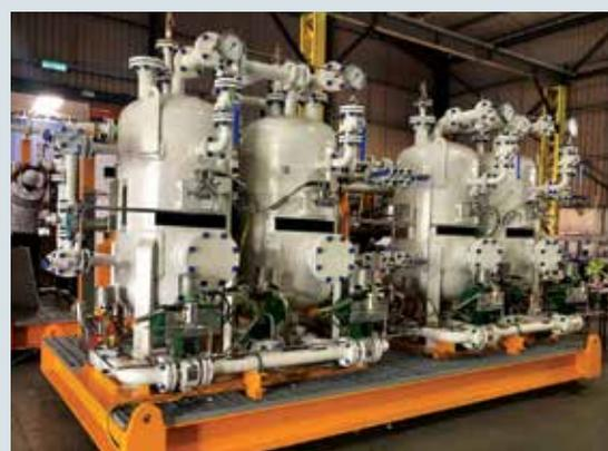
Air Compressor & Air Dryer Package for Pegaga Gas Field
