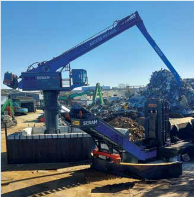
Equilibrium Crane installed at ROMI Recycle, France
